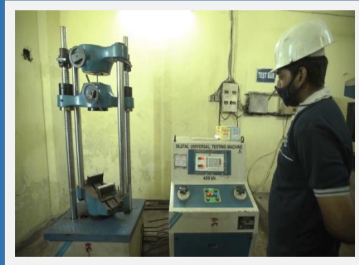
MECHANICAL TESTING OF TEST BAR
