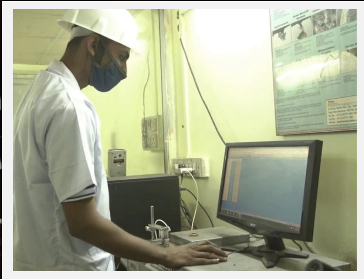
SPECTROMETER For determine chemical analysis of molten metal
