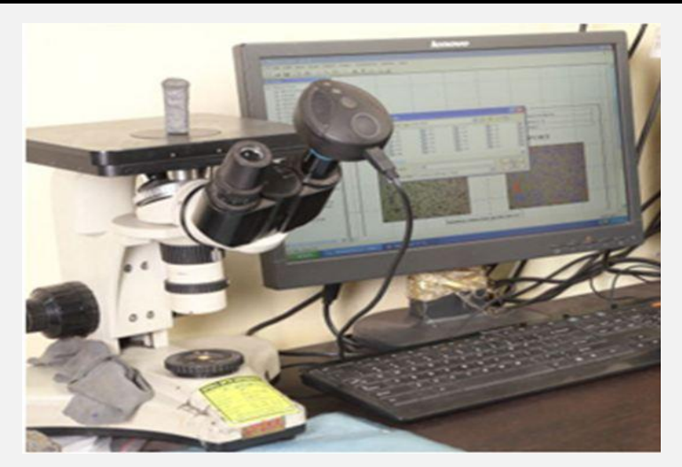
MICROSCOPE With image analyzer for determining microstructure
