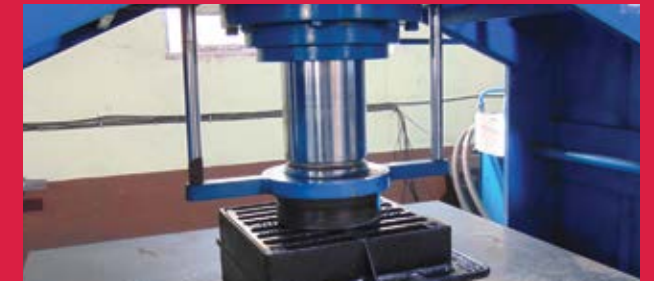
LOAD TESTING MACHINE - With testing facility up to 120 Tons\ 1200 kn
