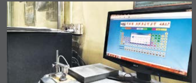
SPECTROMETER - For determining the Chemical analysis of molten metal
