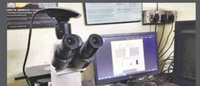
MICROSCOPE - With image analyzer for determining microstructure
